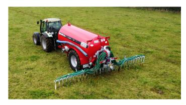
A junction box is attached for rear filling, additional stone collection and splash plating. The box has an outlet underneath for the removal of stones. Large diameter 40mm outlet pipes allow a precise flow of slurry to the lay-flat hosing. The lay flat hosing boasts high ground clearance, which is beneficial over uneven ground.
