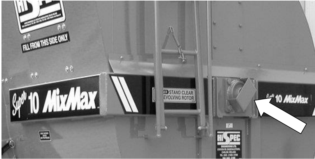
14 Grease Point at Rear of Machine
