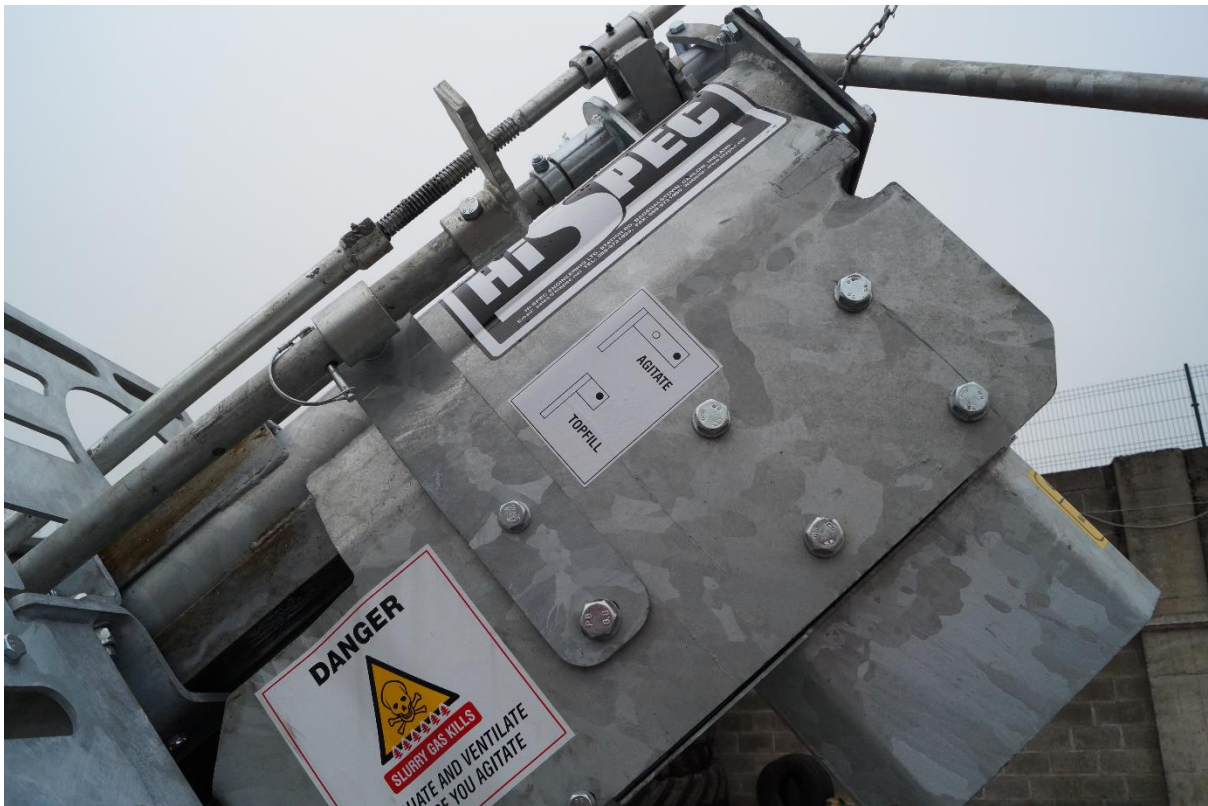
Pump in top fill position.
