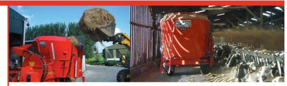
The HiSpec Straw Blower attachment is used for bedding loose and cubicle sheds. It can be used on any size vertical auger machine and will blow straw up to 20 metres to the right hand side of the feeder. You have instant control at your fingertips with all functions operated via an electric controller. Accurate spreading is achieved via adjustment in the two stage chute which will rotate laterally through 30°.
