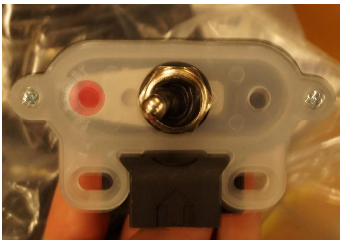
Switch set in macerator / gate position (light is on)
