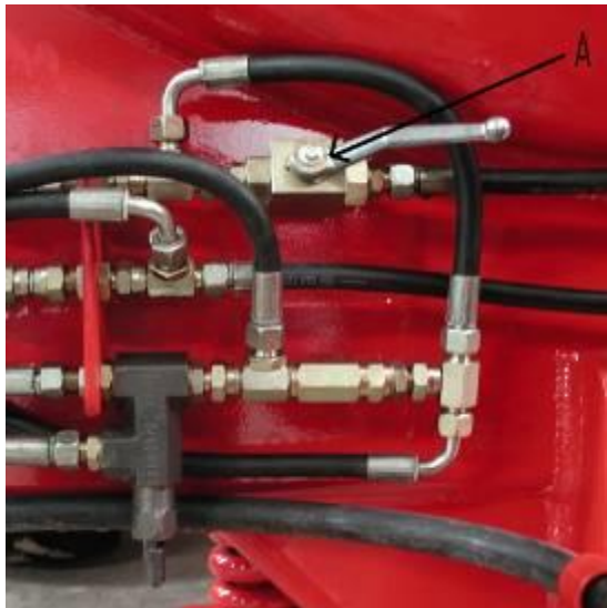
Fig 5: Open/ close valve for boom ram.
